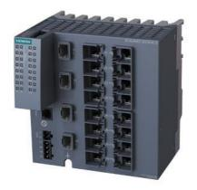
SCALANCE XC216-4C G managed Layer 2 IE switch; IEC 62443-4-2 certified; Full Gigabit; 12x 10/100/1000 Mbps RJ45 ports; 4x 1000 Mbps combo ports (either 1000 Mbps/ SFPs or 10/100/1000 Mbps RJ45 ports can be used); 1x console port; diagnostics LED; redundant power supply; temp. range -40 °C to +70 °C; mounting: DIN rail/S7 mounting rail/wall; redundancy functions; Office features (RSTP, VLAN,...); PROFINET IO device; Ethernet/IP-compliant; C-plug slot;
